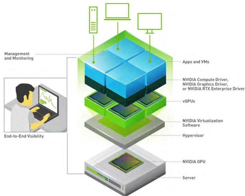
NVIDIA vGPUs are comparable to conventional GPUs in that they have a fixed amount of GPU Memory and one or more virtual display outputs or *heads*. Multiple heads support multiple displays. Managed by the NVIDIA vGPU Manager installed in the hypervisor, the vGPU Memory is allocated out of the physical GPU frame buffer at the time the vGPU is created. The vGPU retains exclusive use of that GPU Memory until it is destroyed.
