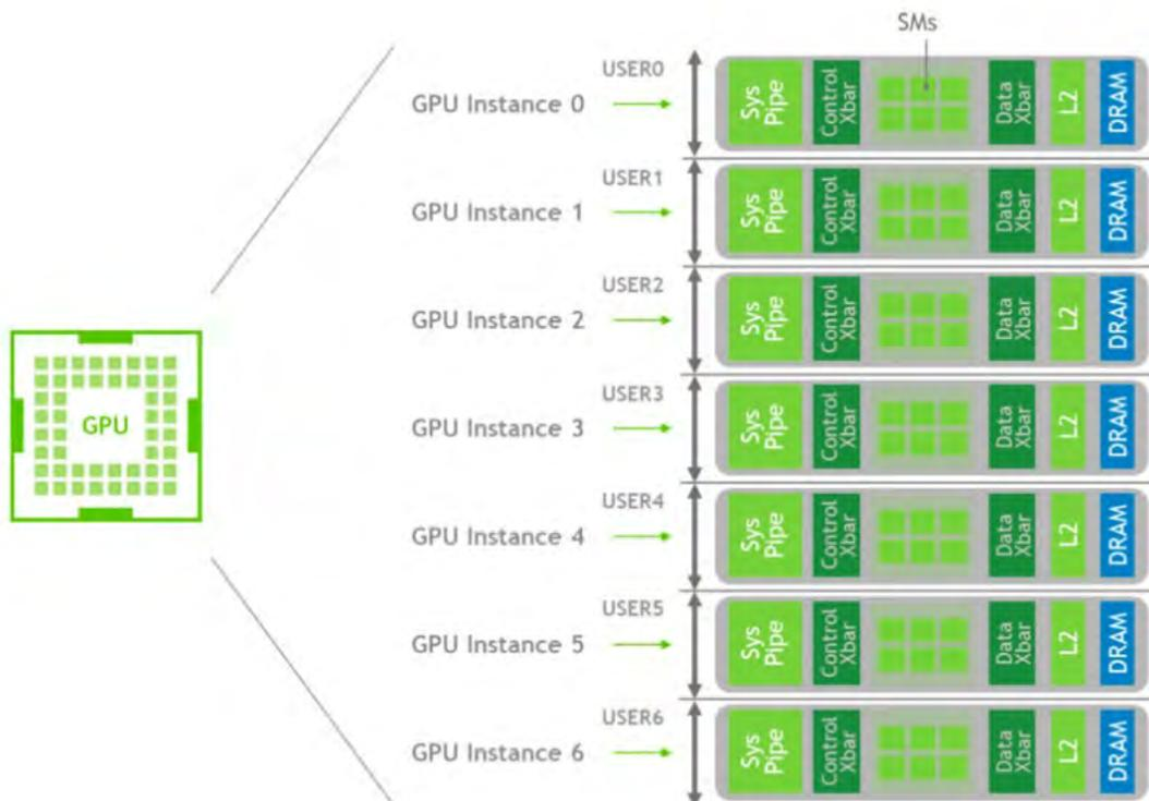
Each instance’s processors have separate and isolated paths through the entire memory system. The on-chip crossbar ports, L2 cache banks, memory controllers, and DRAM address busses are all assigned uniquely to an individual instance. This ensures that an individual user’s workload can run with predictable throughput and latency, using the same L2 cache allocation and DRAM bandwidth, even if other tasks are thrashing their own caches or saturating their DRAM interfaces.
